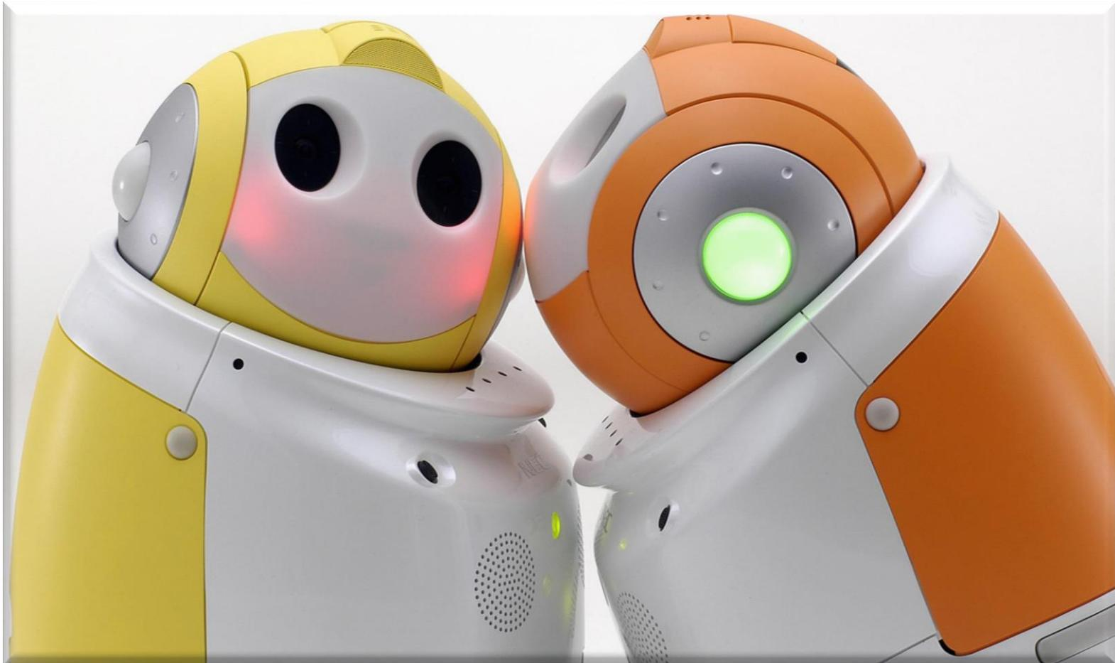
*Equipped with light, audio, temperature, posture, motion, audio sensors, face recognition, voice recognition and behavior detection.*
